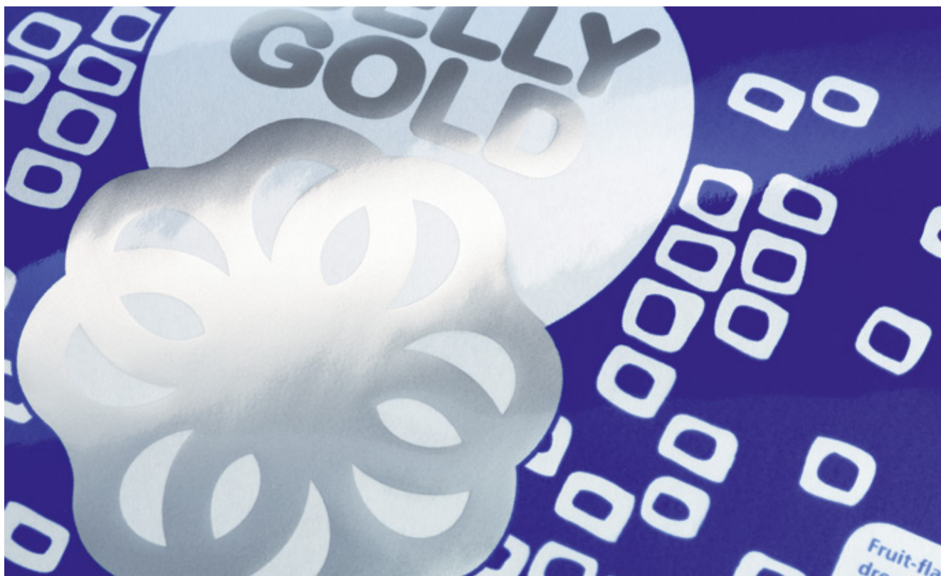
Reverse, gravure print onto film – silver effect based on ROTOVARIO Pigment Paste/ 薄膜凹版里印 - 基于 ROTOVARIO 铝浆的银色效果
